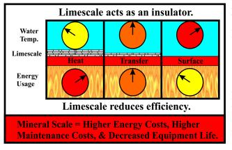
Mineral scale deposits in water-fed equipment cause many problems. In water heating equipment, scale builds up in layers on heat transfer surfaces, insulating water from efficient heat transfer resulting in higher energy costs. Scale build up also increases maintenance costs and decreases equipment life.
