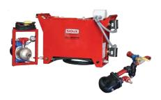
The Sioux Condensate Return System is a portable accessory that turns the standard Steam-Flo® steam generator into a closed-loop system. By collecting and recycling the condensate and water used during steam heating, the Condensate Return System:
